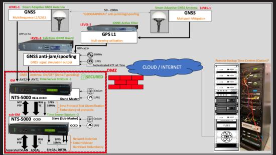
NTS-5000 NTS-Smart-antenna SafeTime GNSS guard GPS L1 active filter
