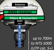
Easy GNSS receiver replacement enables customized cybersecurity. It also ensures correct industry profile settings suitable for a region's current "geopolitical" situation. Protection of the input time from GNSS source has become increasingly important today, and therefore, it requires flexibility in changing to GNSS trusted receivers.
