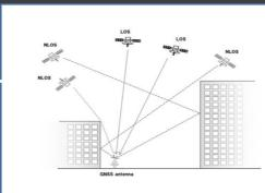
Optionally, customers can request a particular GNSS cyber-security receiver version made by Furuno, who has developed a new unique technology to enhance the reception of GNSS signals. This unique functionality enables correct timing signals to be computed even when antennas are mounted in a lower part of the canyon, where GNSS signals are reflected, diffracted, jammed or spoofed.
