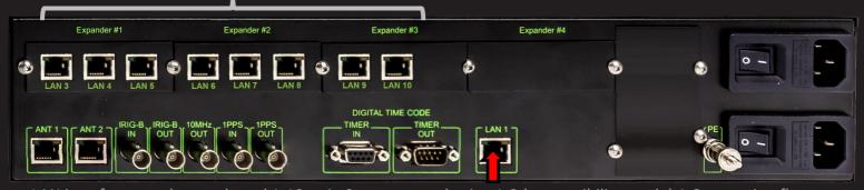
LAN interfaces can be numbered 1-10 or in 2 groups numbering 1-2 (compatibility mode) 1-8 extension floor
